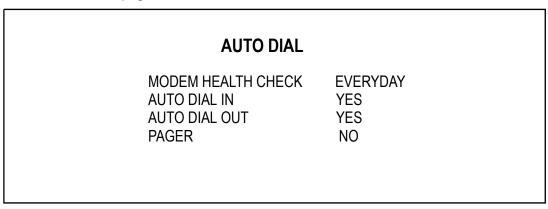
The settings for Modem Health Check, Auto Dial In, and Auto Dial Out, can be changed by highlighting the item and pressing SELECT, which will bring up the appropriate screen
